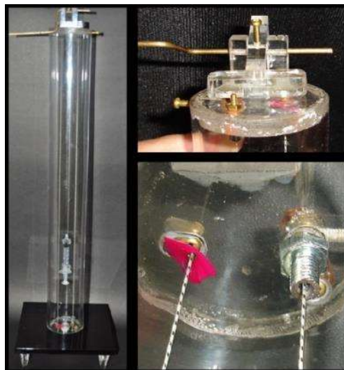
Figure 3. Showing the vacuum chamber made from a transparent plastic tube with outlet for air with a valve and magnetic holding lever.
